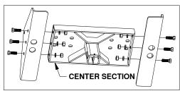
Figure A1: Underside view of center section and legs.
