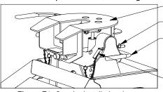
Figure E1: Coupler installed on base.
